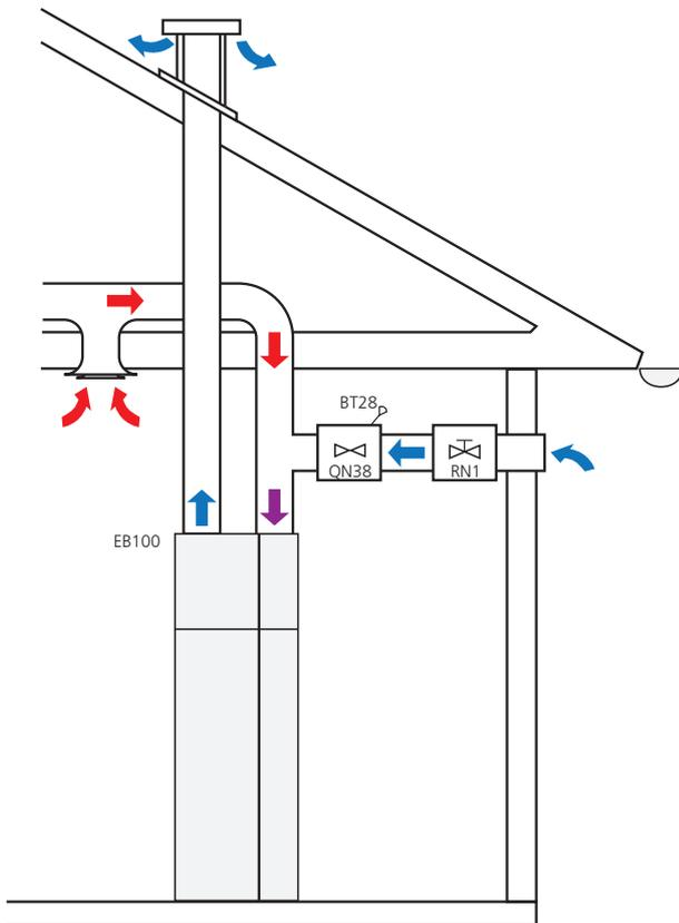
The hot air is transferred from the rooms to the heat pump (EB100) via the building's ventilation system.
