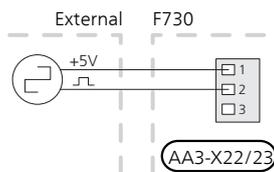
Activate the energy meter(s) in menu 5.2.4 and then set the desired value (energy per pulse) in menu 5.3.21.
