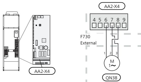
The switch for the direction of rotation of the motor is set at the factory as below.
