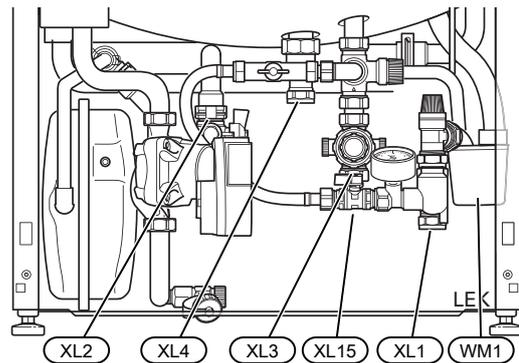
The overflow cup (WM1) can be turned, so that the pipe can be directed forwards or backwards to simplify connection of the hose to the drain.
