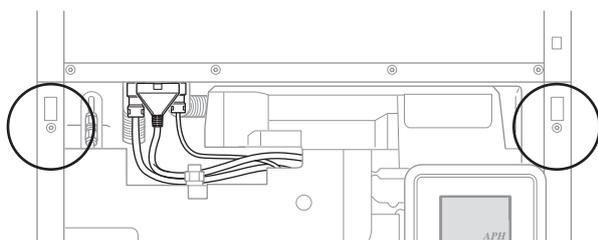
11. Secure the air treatment unit lock tabs in the water heater unit with 2 of the screws supplied.
