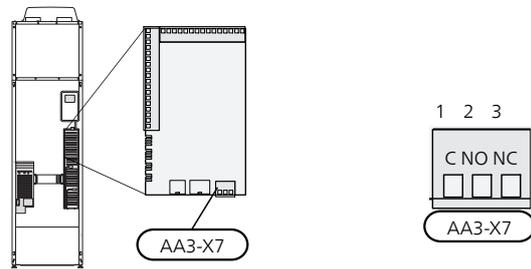
The picture shows the relay in the alarm position.
